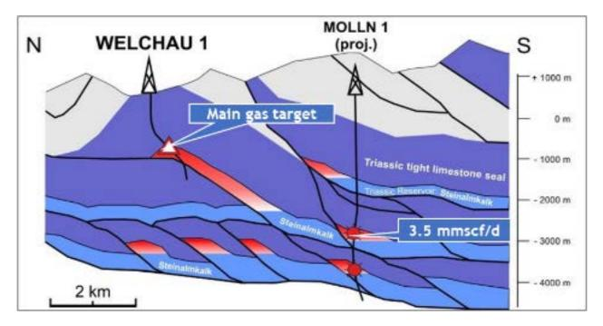
Figure 4: Schematic cross section of the Welchau gas prospect and the Molln-1 gas discovery.
