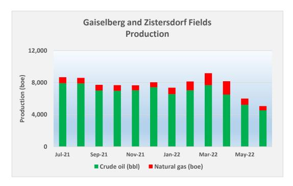
Production histogram showing the production drop in May and June due to well down time
