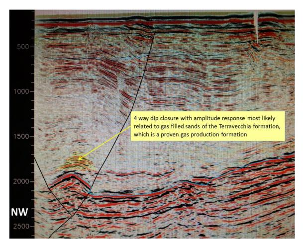
2D seismic line showing in yellow the bright amplitudes of the Terravecchia (Miocene) sandstones draping an underlying Nilde formation oil prospect
